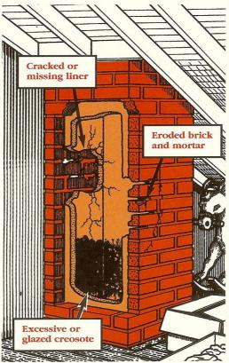
When we look at the interior of this same chimney we can find a number of imperfect conditions. Pieces are missing from the original clay liner and there are cracks in the clay liner. (Old chimneys might not even *have* a liner.) Mortar and bricks are loose and falling. And there is excessive buildup of combustible creosote on the flue walls.
